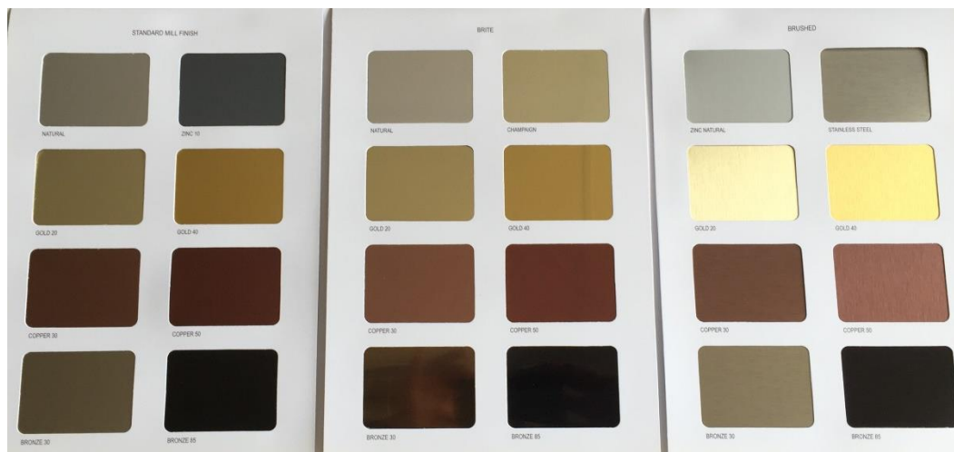
Figure 8.1: Example of pallet of colours from anodization process (Coil, Aloxide products)
