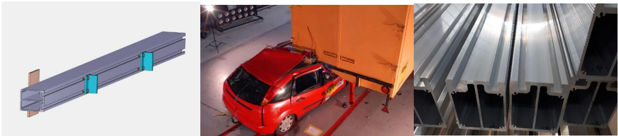
Figures 10.37, 10.38 and 10.39: Rear underrun protection component, car intrusion test, aluminium beams (pictures by Hydro)
