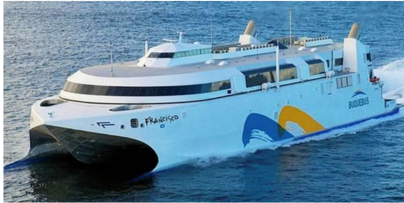
Figure 2.5 - The world's largest aluminium boat, 130m long and 32m wide
