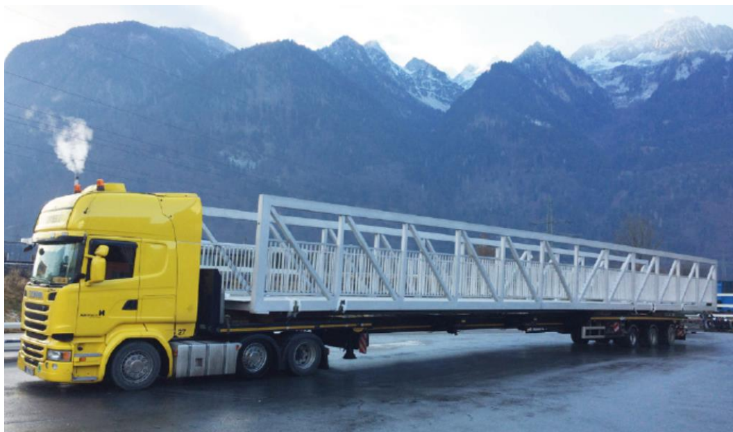
Figures 4.3 and 4.4: Examples of transportation of fully prefabricated structures.
